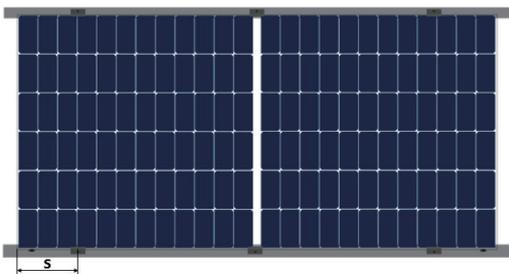
Installation of frameless module with fixtures on long sides
