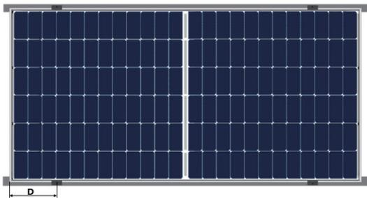
Installation of framed module with fixtures on long sides (beam parallel to long sides)
