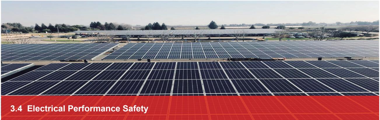
PV modules can produce DC current under illumination, any contact of the exposed metal of the modules connection wires may result in electrical shock or burn. Any contact of 30V or larger DC Voltage can be fatal.
