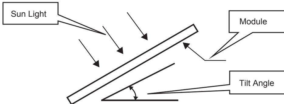
Modules are preferred to be south-facing in the north hemisphere and north-facing in the south hemisphere. Please refer to standard modules installation guideline or suggestions from experienced PV module installer, for the specific installation angle.
