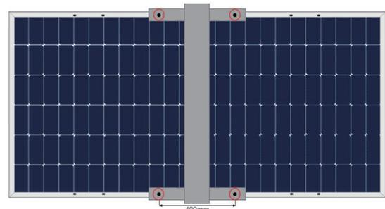
Installation with bolts into 400mm-span holes
