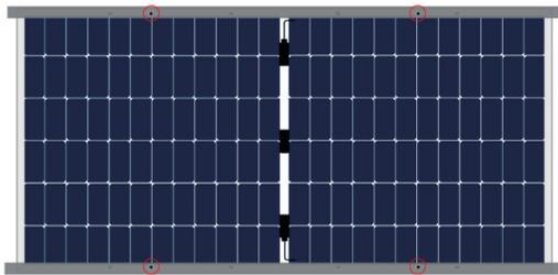
Installation with bolts into 4 inner holes
