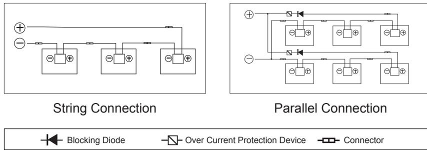
Figure 10 Series Connection and Parallel Connection Circuit Diagram
