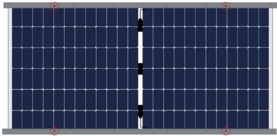
Installation with bolts into 4 outer holes
